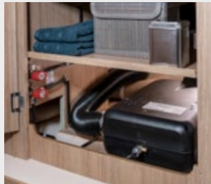
"Truma VarioHeat Eco" gas heating (only TRAIL/BOX 200)
