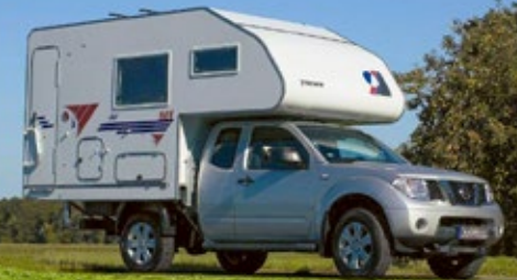
BOX 260S on Nissan Navara, platform flatbed with fold-down, detachable tailboards
