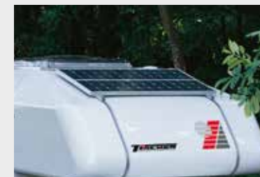
100 Watt solar system, charge control
