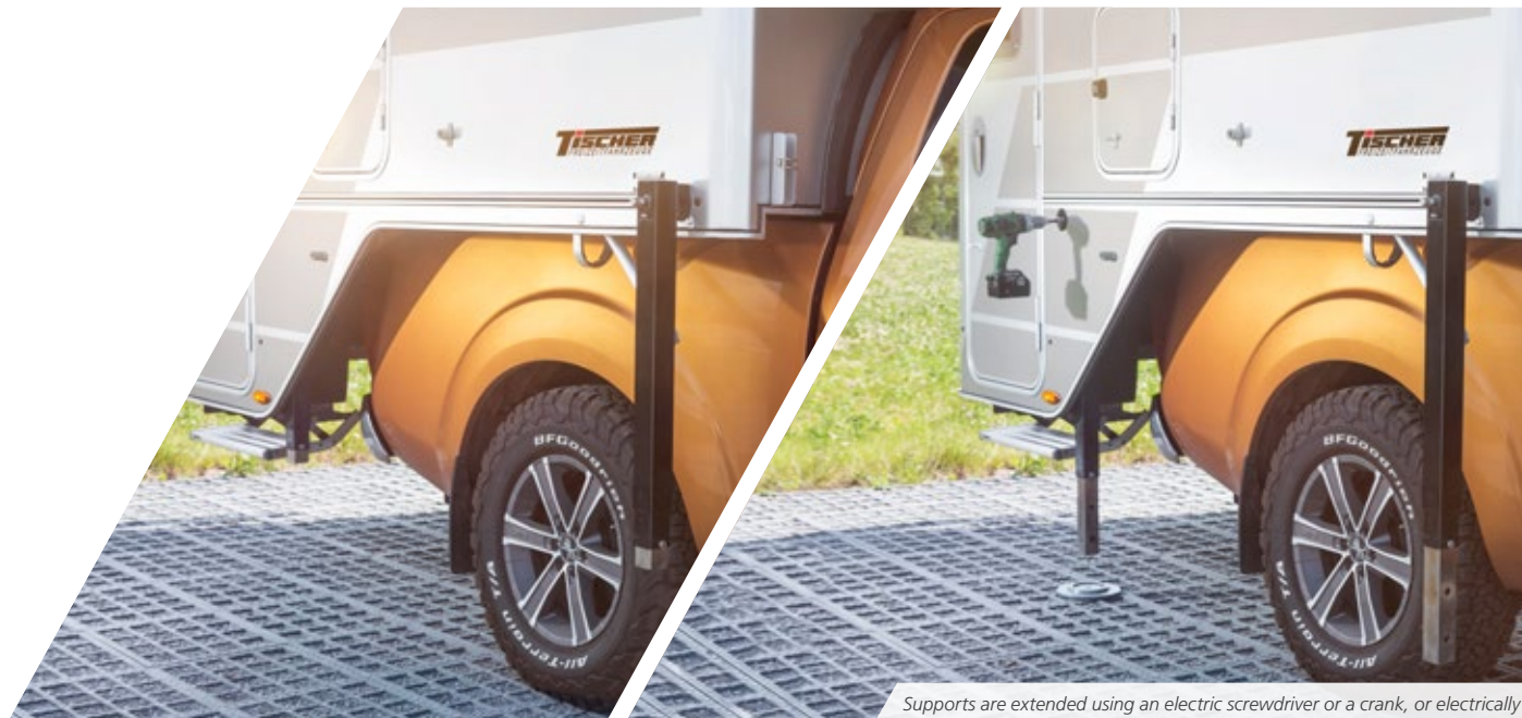
Supports are extended using an electric screwdriver or a crank, or electrically
