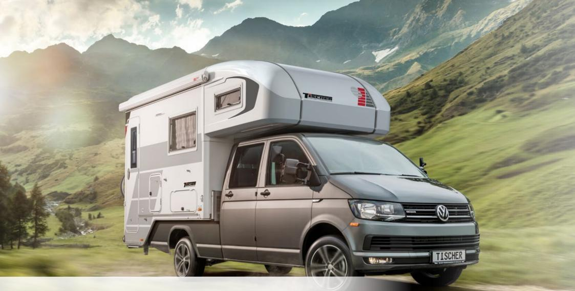
The TRAIL/BOX 280 cabin model (with back entrance) and the 280S and 285S models (both with side entrance) were specially designed for VW flatbed trucks.
