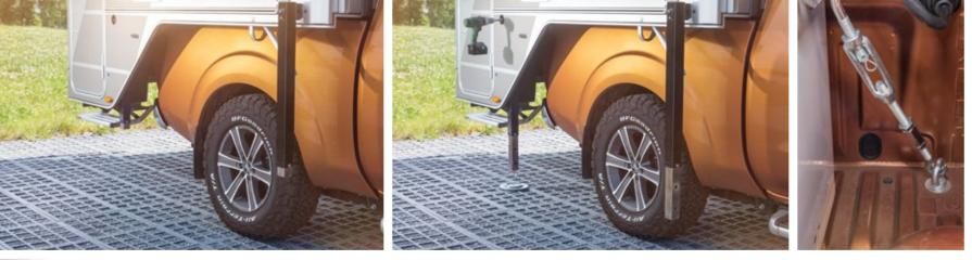
Extend supports with cordless screwdriver or crank handle
