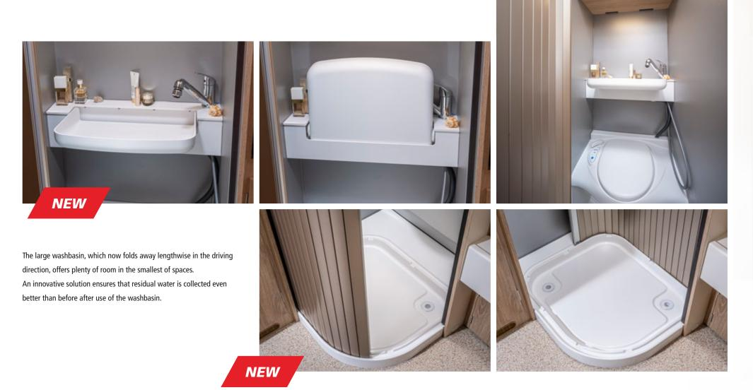
The guide of the shower door has been optimized to use up less living space when the bathroom is not in use.
