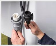
13-pin plug for lighting and 3-pin high-current plug for battery charging
