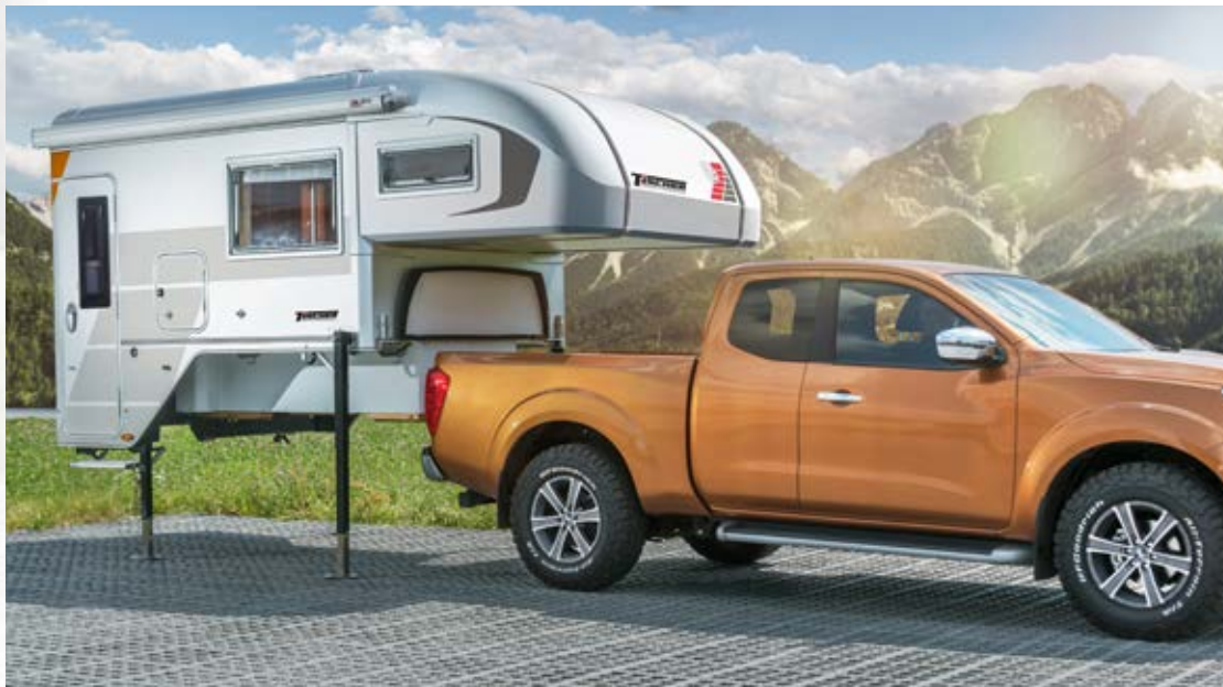
Extend supports with cordless screwdriver or crank handle
