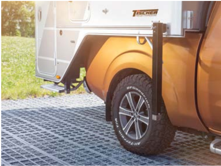
Extend supports with cordless screwdriver or crank handle
